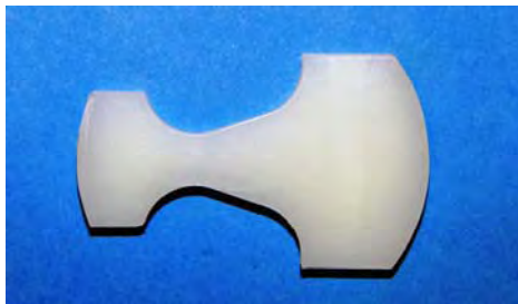
Figure 1. Constant stress specimen
