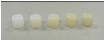
Figure 1. UHMWPE Pins (left to right) Virgin, 300 ppm VE, 1000 ppm VE, 1000 ppm 5 MRad and 1000 ppm 10 MRad.
